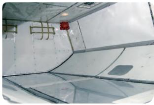
Flame-retardance, high tensile strength, and excellent puncture and tear resistance are required for seaming, patching, and repairing panels in aircraft cargo compartments.
